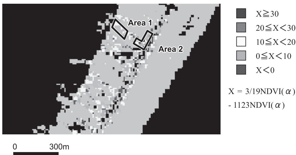
Figure 7. Level of the 19 March-23 Nov NDVI differences on the 'No damage' coastal forest area after the tsunami.
