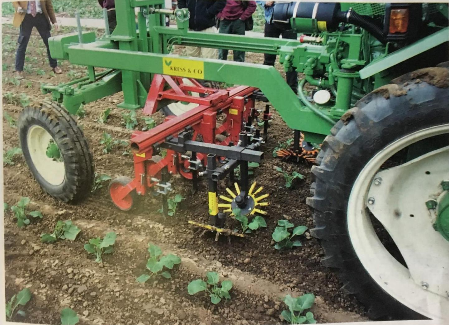
Fig 29 Finger weeder mounted on specialist weeding machine.
