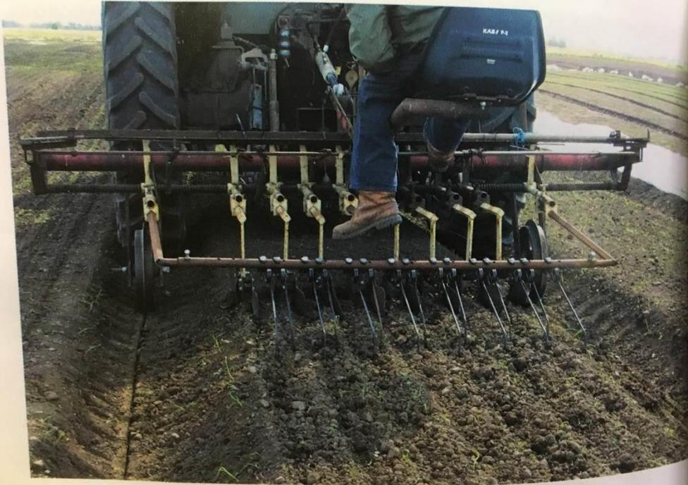
Fig 30 A home-made torsion weeder.
