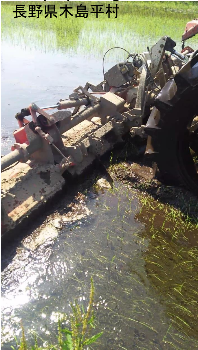
Weeding by deep water shallow plowing Nagano kijimadaira 深水代掻き除草
