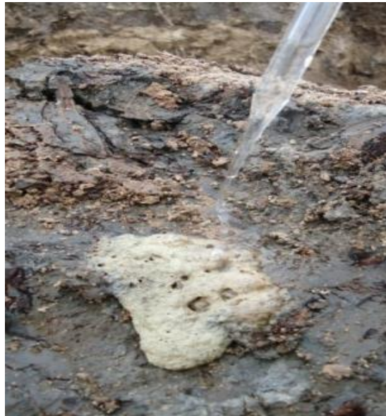
Gray colored, reaction with \text{H}_2\text{O}_2 will be effervescent
